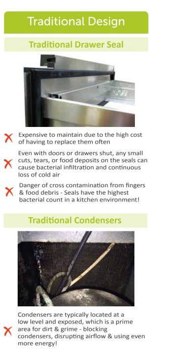
Unless brush cleaned often, airborne contaminants, such as fat & flour, clog up the condenser, burning out fan motors and even compressors
