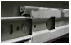
Drawer runners must be fixed into the insulated cabinet wall, making them х inherently weak, and in need of frequent replacement
