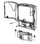
Refit the front cover and secure with 2 fixing screws. Close the dosing unit door.
