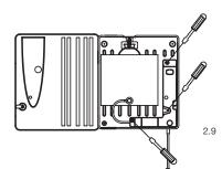
Refit the electronics cover. Check the fluid box can move up and down freely. Close the dosing unit door.
